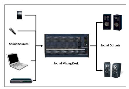
Unlike a hi-fi which just has one volume control for everything, a sound mixing desk normally allows you to separately set the volume or level of each source and the level of each output. However, in order to hear a sound out of the speakers, the levels must be turned up for both sources and outputs.
