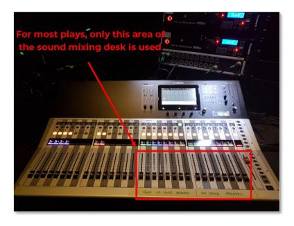
The most confusing concept for any new operator of a sound mixing desk will be the idea of dealing with both inputs and outputs. A sound mixing desk is designed to combine or "mix" together the sound from various inputs or sources (such as CD players, MP3 players or laptops) into an array of different outputs (such as speakers).
