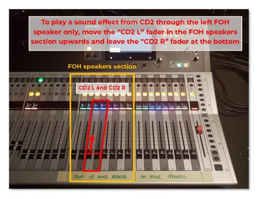
For example, if you are playing a sound from the CD2 player, to hear the sound from the left FOH speaker as you look at the stage, only move up the "CD2 L" speaker fader in the FOH speaker section and leave the "CD2 R" fader at the bottom of the scale.
