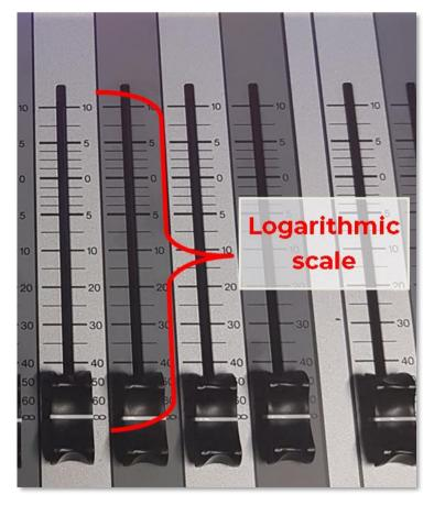
f) As an example of setting the faders, to hear music from the CD1 player out of both left and right FOH speakers, the two faders for the CD1 player within the section for the FOH speakers should be pushed upwards.
