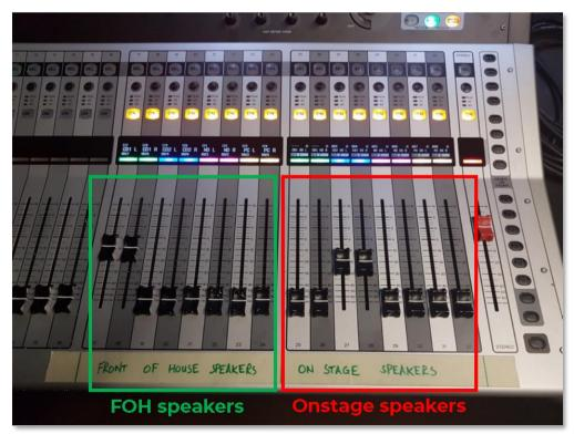
c) Within each area for each set of speakers, there are two faders for each input or source (such as each CD player) – one controls the sound on the left side and one the sound on the right. The small screen above each fader indicates which source and which side of the stage the fader relates to. There are faders for the CD1 and CD2 players and for the two 3.5mm jack audio cables (for use with laptops and digital media players and labelled "PC1" and "PC2").
